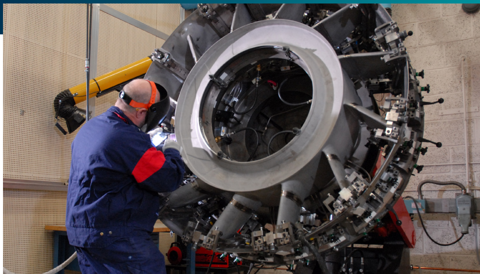
Welding of a turbine rear frame in GKN Aerospace's Kongsberg plant.
